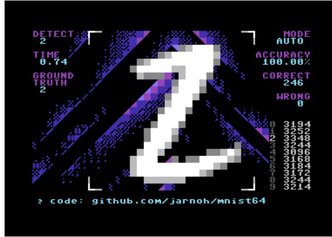
Figure 2: C64 running the MNIST64 program, with visuals and inference details. Digits are streamed from a floppy disk (6 disksides for 10,000 digits). Correct detections are indicated with digitized voice samples.
